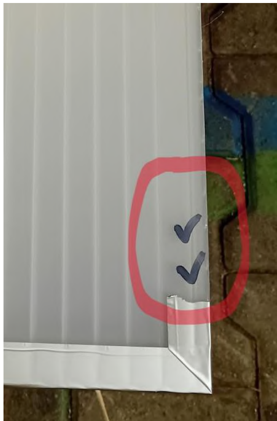
Figure 38 Method of marking the UV-resistant side of polycarbonate sheets.
